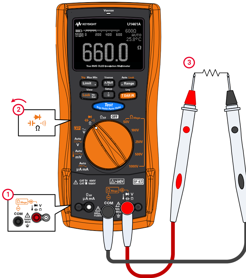
Figure 2-16 Resistance measurement example
